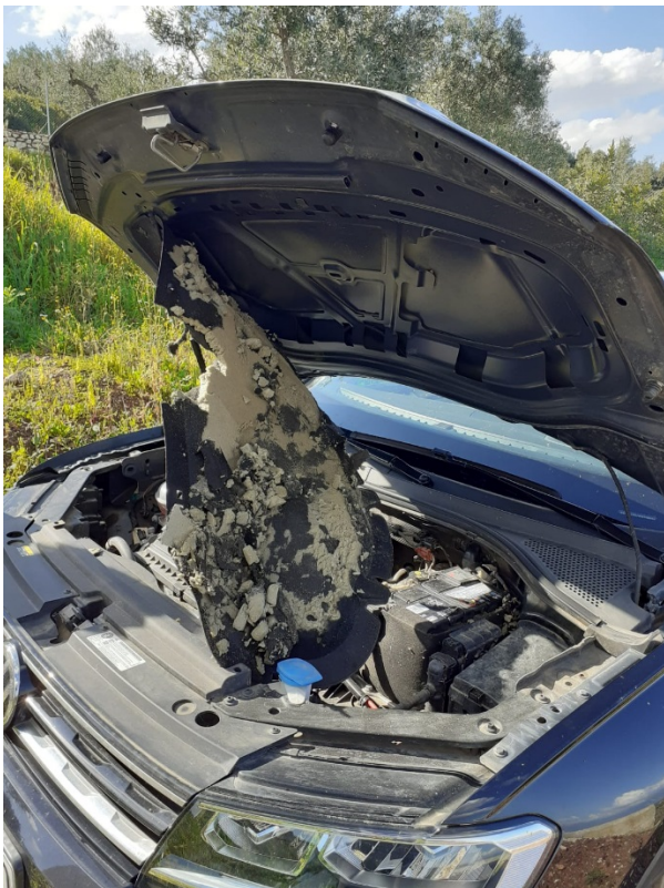
Pine marten damage under the bonnet.
